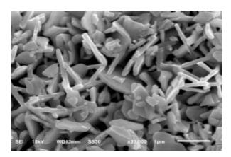
Figure 3: SEM micrographs of  $Sr_{1-x}Bi_{3+x}LaTi_{4-x}Mn_xO_{15}$  with x = 0.6 synthesized by hydrothermal technique.
