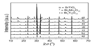
Figure 1: X-Ray Diffraction (XRD) patterns of Aurivillius phases Sr<sub>1-x</sub>Bi<sub>3+x</sub>LaTi<sub>4-x</sub>Mn<sub>x</sub>O<sub>15</sub> were synthesized by hydrothermal technique. a) SrBi<sub>4</sub>Ti<sub>4</sub>O<sub>15</sub> [11], b) x = 0, c) x =0.2, d) x = 0.4, e) x = 0.6, f) x = 0.8, g) x = 1.
