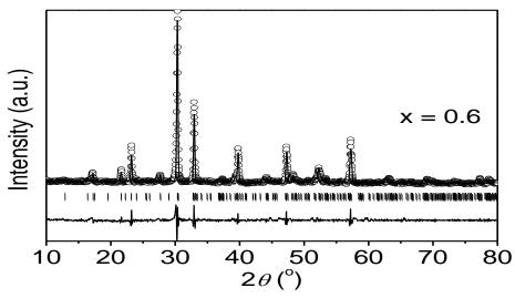
Figure 2: Le Bail plot of XRD powder of  $Sr_{1-x}Bi_{3+x}LaTi_{4-x}Mn_xO_{15}$  with x = 0.6 synthesized by hydrothermal technique. Observed XRD intensity (circle), calculated data (solid line), and the difference of patterns,  $y_{obs} - y_{cal}$  (solid line on the bottom curve). The tick marks represent the positions of allowed Bragg reflections in the phase of  $A2_1am$ .
