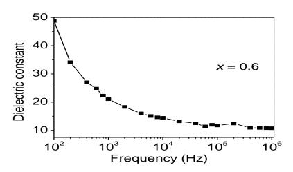
Figure 4: Frequency dependence of dielectric constant of  $Sr_{1-x}Bi_{3+x}LaTi_{4-x}Mn_xO_{15}$  with x = 0.6 synthesized by hydrothermal technique.
